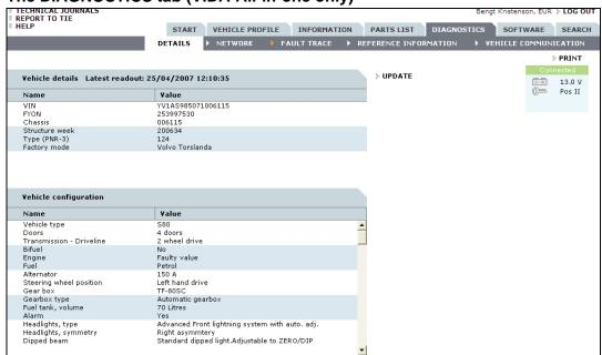
To use VIDA diagnostics, a vehicle must be connected to the communication tool VCT2000 or DiCE.
