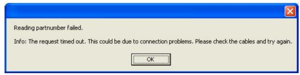
2. If the part number of the software can not be read, the application will display an error message, see above. To update the control module when this has occurred
