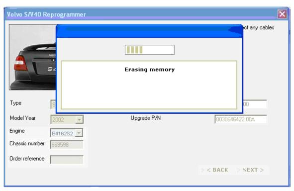
12. When the application has opened the control module, the download procedure starts.
